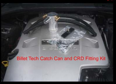
Screw catch can to fixing bracket and 'dry fit' to ascertain and mark fitting position with engine cover in place
