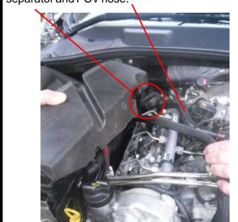
Locate oil separator to the rear of the bulkhead and remove via 3 torx head bolts.
